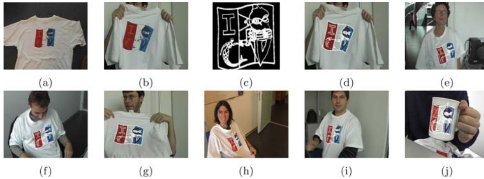
Figure 1. In order to achieve surface detection, we use a model image (a). Then, our method computes a function mapping the model to an input image (b). To illustrate this mapping, we find the contours of the model using a simple gradient operator and we use them as a validation texture (c) which is overlaid on the input image using the recovered transformation (d). Additional results are obtained in different conditions (e to i). Note that in all cases, including the one where the T-shirt is replaced by a cup (j), the white outlines project almost exactly to the right place, thus indicating a correct registration and shape estimation. The registration process, including image acquisition, takes about 100 ms and does not require any initialization or a priori pose information.
